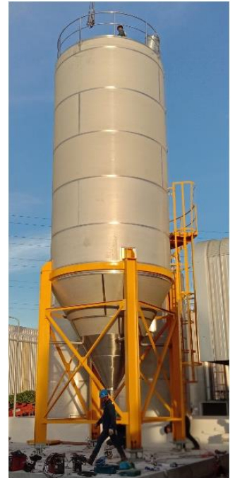
Stainless steel 304 PVC Resin Silo, Size 100 m 3
