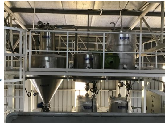
Stainless steel 304 PVC Resin Silo, Size 100 m 3
